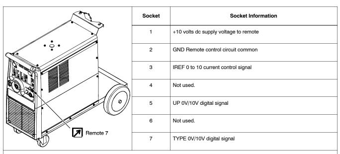
Note: This remote receptacle cannot be used with a standard Miller remote control. A customer supplied remote control is required to use the remote receptacle.
